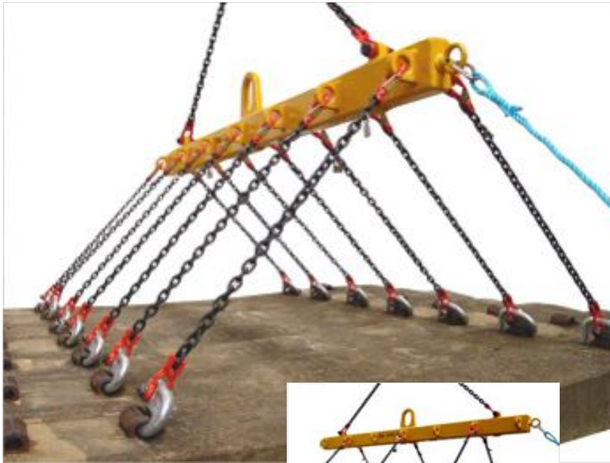
Inset shows a 7 sleeper lifting beam used to lay 3 sleepers.
