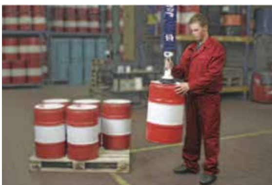
JumboFlex, maximum load 35kg, with round suction pad for handling barrels
