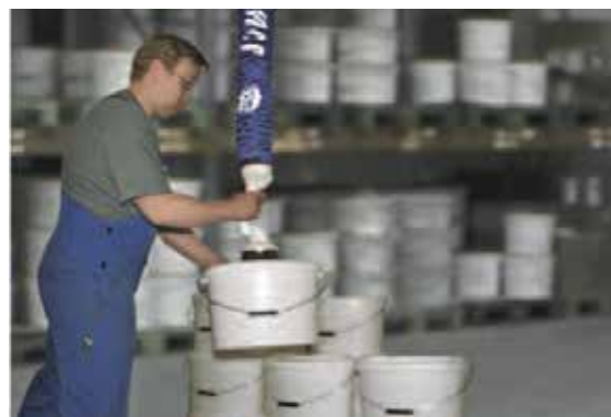
JumboFlex, maximum load 35kg, with round suction pad for handling buckets
