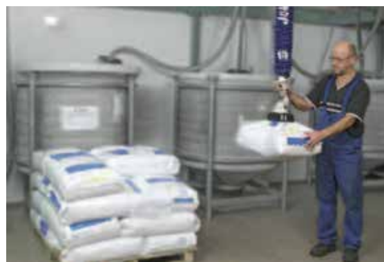
JumboFlex, maximum load 35kg, with sack suction pad for handling sacks
