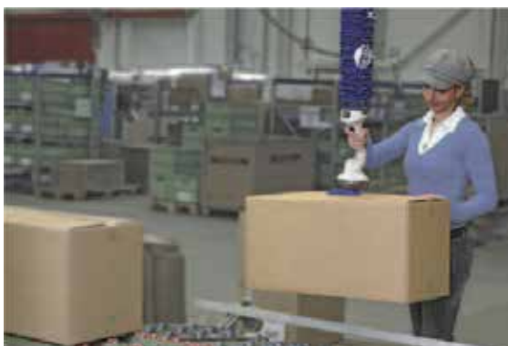
JumboFlex, maximum load 35kg, with double suction pads for handling cardboard boxes
