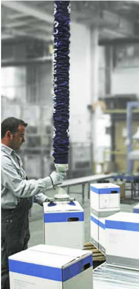
JumboFlex, maximum load 35kg, with double suction pads for handling cardboard boxes in the shipping area
